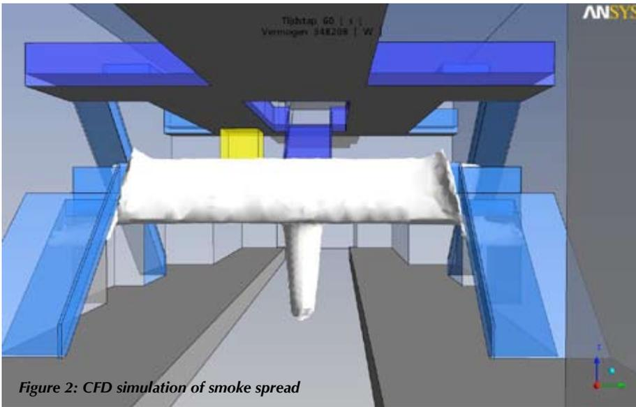
Figure 2: CFD simulation of smoke spread
